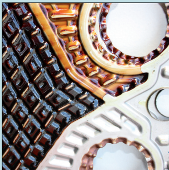
Varnish on plate heat exchanger
