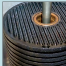
Varnish Removal insert, VRi, after filtration
