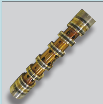
Varnish on valve spool
