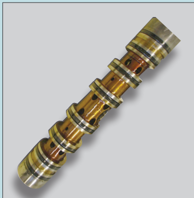
Varnish on valve spool
