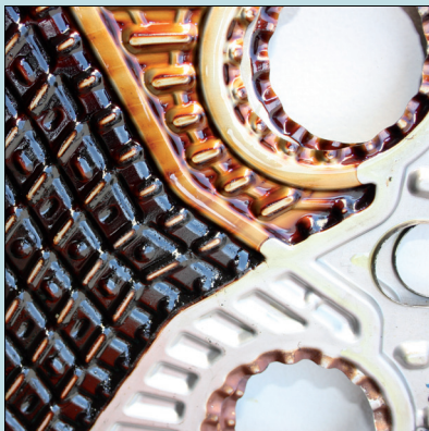
Varnish on plate heat exchanger
