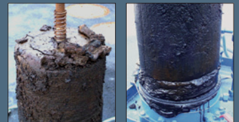
approx. 30 kg of dirt after 6 weeks of filtration
