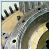
Pitting on bearing
