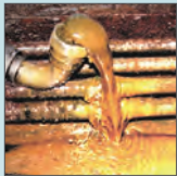
Water Contaminated Oil
