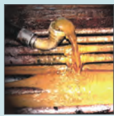
Water contamination on steel mill/ gear
