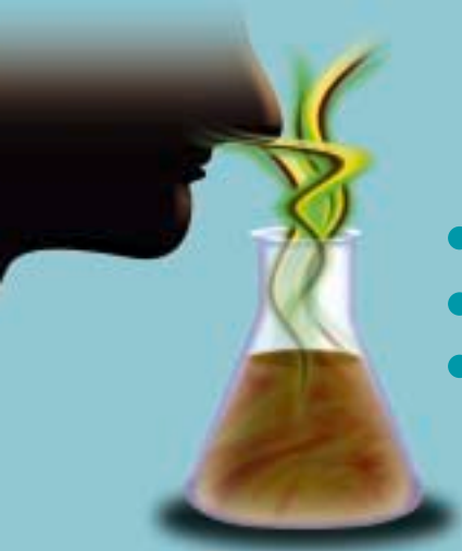
Sour and putrid odor indicates oil degradation
