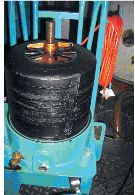
CJC™ FilterInsert A27/27 - After test.
