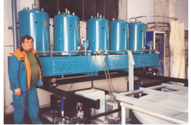
Mr. Pekka Korhonen at Metso Drives Oy, with the HDU filtration unit for their 90,000 litre system.
