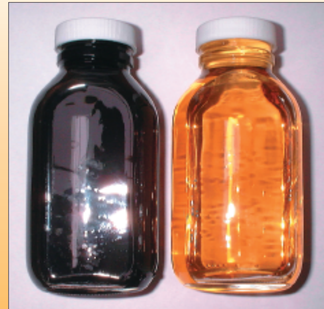
Tap changer oil without and with continuous use of CJC™ Fine Filter
