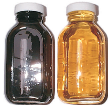
Oil samples - before and after filtration.
